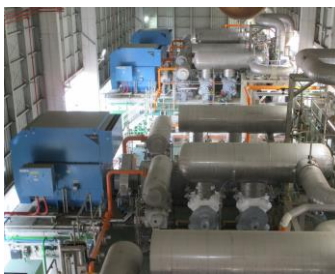
HP LP Reciprocating compressors, Fluxys, Bélgica
